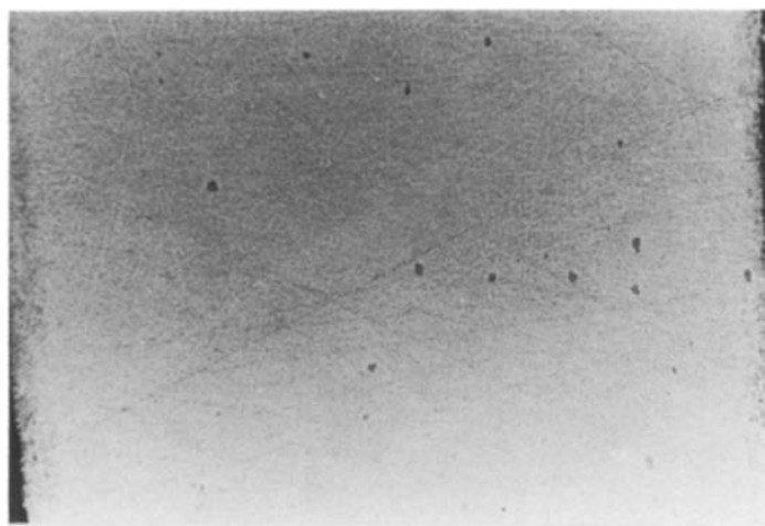
Figure 5 Optical micrograph of Zn–Al eutectoid deformed superplastically to 400 pct. elongation at 250°C (0.7 Tm), strain rate = 1.6 \times 10^{-3} \text{ sec}^{-1} . There is little cavitation. The \text{FeAl}_3 type inclusions are shown. Tensile axis is vertical. ( \times 140 )
